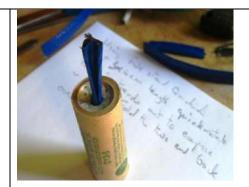
Place the motors with QM attached into the rocket. Connect the motors together by using tape match folded over each QM with a single igniter at one end of the tape.
