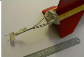
As before, three quick matches are inserted into the motors. This time the matches are connected to the igniter using tape match.
