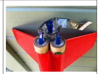
Alternatively: Three single strands of quick match are inserted into the motors and held firm in place using masking tape. The matches are brought together and taped to a single Estes igniter. Note: the ends of the QM in the motor are folded over to improve the reliability
