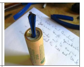
Place the motors with QM attached into the rocket. Connect the motors together by using tape match folded over each QM with a single igniter at one end of the tape.
